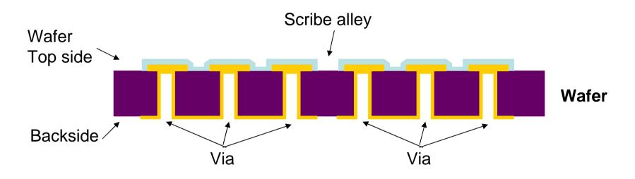
Backside via process is the process to make the via to connect all the ground/source in an IC together. The via metal is made of plated Au.
